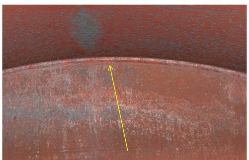
Fig 3. Closer view of front tubeplate to shell showing two off 2 mm diameter holes at the tubeplate toe of the internal fillet weld.
